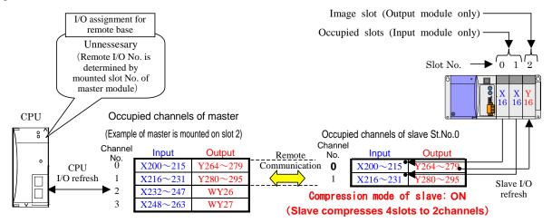
Figure 4.6 Correspondence of occupation channels and I/O slots in slave with compression mode (4W/4W method)
