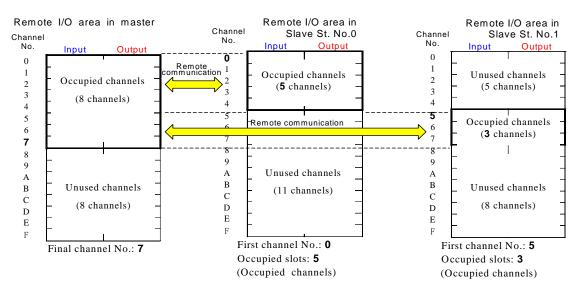
Figure 4.4 Occupied channels and remote communication
