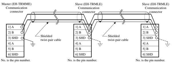
Figure 5.6 Connection method when enabling the replacement of slave module while operating
