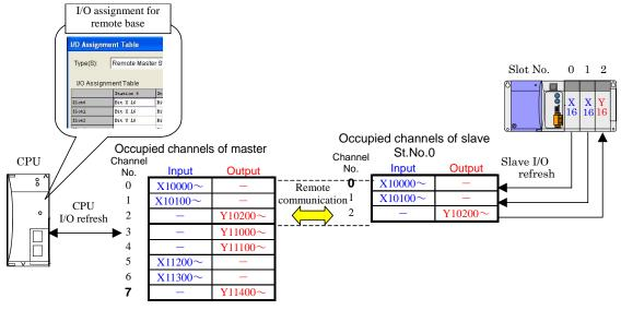
Figure 4.5 Correspondence of occupied channels and I/O slots
