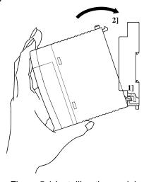
Figure 5.1 Installing the module
