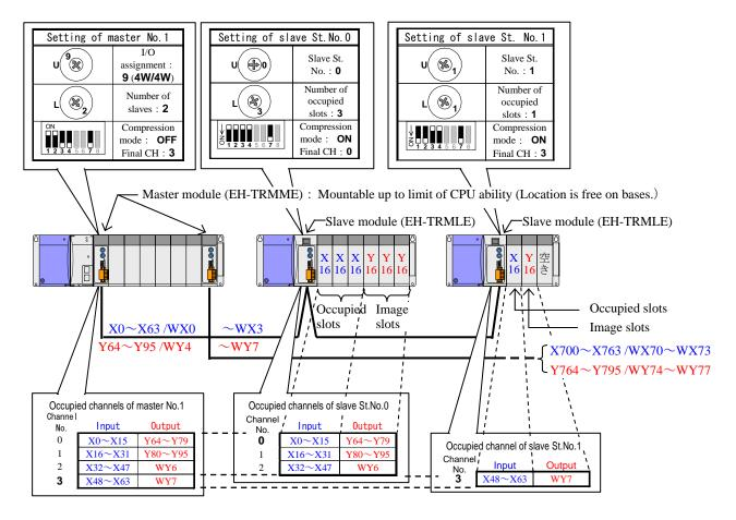
Figure 4.12 System configuration example-1 (I/O assignment of master: "Word 4W/4W")
