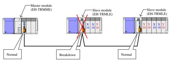
Figure 6.2 Fallback operation when breakdown in slave module occurs
