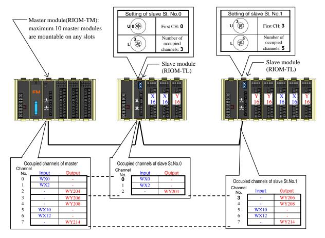
Figure 4.32 System configuration example-15 of the EM/EM-II series (Not using image slot)
