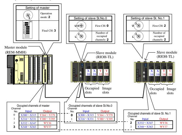
Figure 4.24 System configuration example-9 of Remote I/O MINI with mode-2
