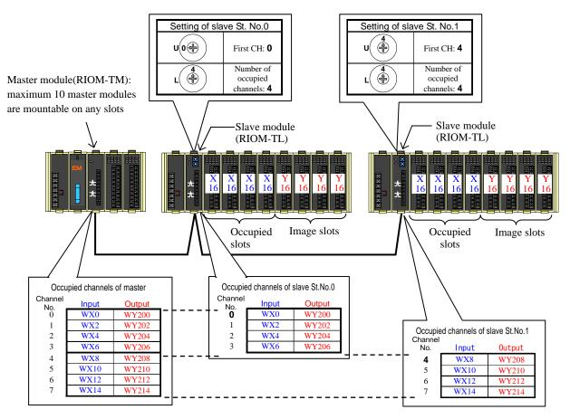
Figure 4.35 System configuration example-17 of the EM/EM-II series (Using image slot)
