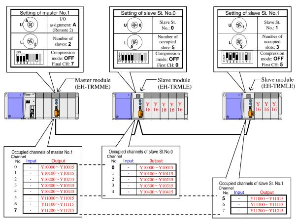
Figure 4.22 Replaced system configuration example-8 of the EH-150
