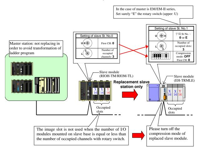
Figure 4.38 Replacement of only slave station in the case of using no image slot (compression mode: OFF)
