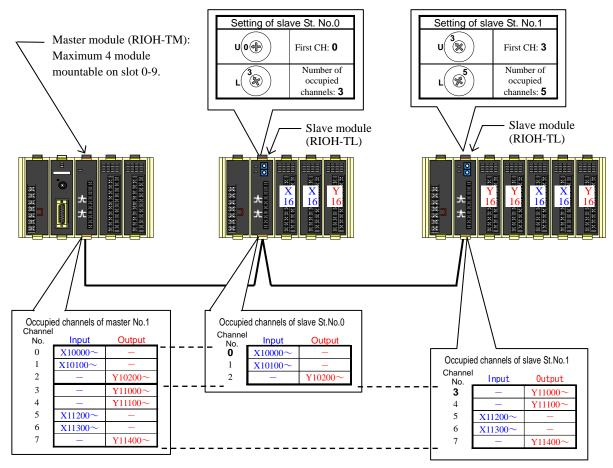
Figure 4.15 System configuration example-3 of the H-200 series (Not using image slot)
