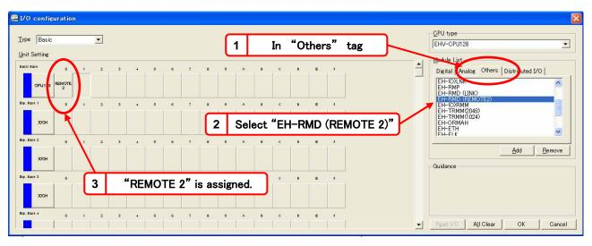
Figure 1.1 I/O assignment for remote master with control editor of unsupported version (in the case of "REMOTE 2")
