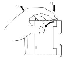
Figure 5.2 Removing the module
