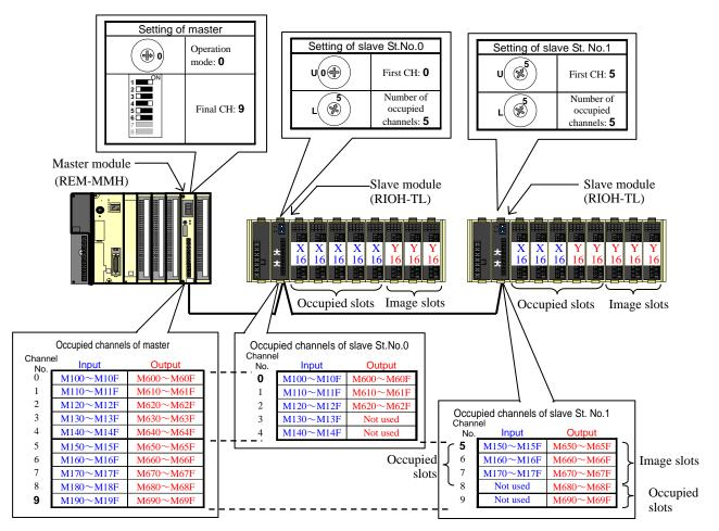
Figure 4.29 System configuration example-13 of Remote I/O MINI with mode-0
