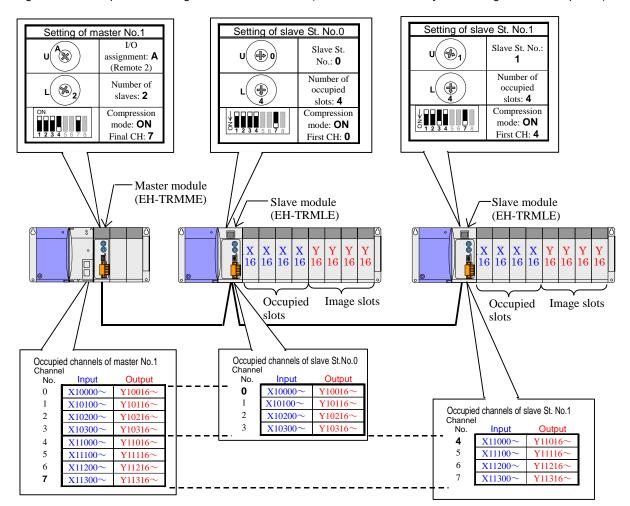
Figure 4.37 Replaced system configuration example-18 of the EH-150 (Using image slot)
