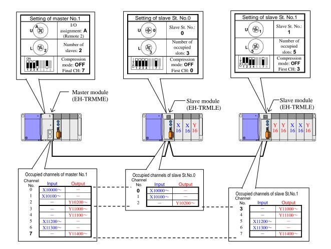
Figure 4.17 Replaced system configuration example-4 of the EH-150 (Not using image slot)
