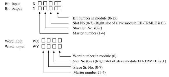
Figure 4.10 I/O number of I/O module on remote slave base
