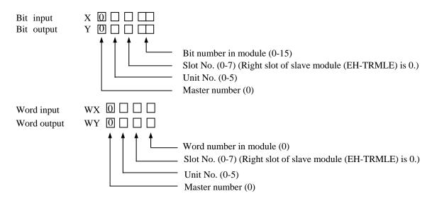
Figure 4.13 I/O number of I/O module on remote slave base (I/O assignment for master: "Word 4W/4W")
