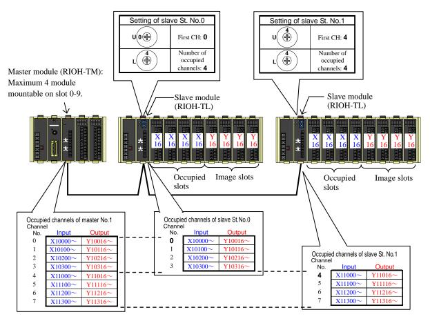
Figure 4.18 System configuration example-5 of the H-200 series (Using image slots)
