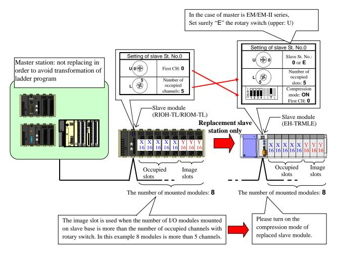
Figure 4.39 Replacement of only slave station in the case of using image slot (compression mode: ON)
