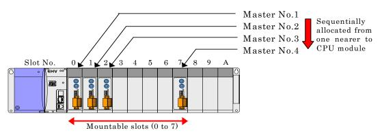
Figure 4.2 Mountable slots for master module and master number
