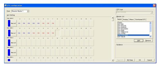
Figure 4.30 Example of I/O assignment for slave bases (with Control editor in system configuration example-14)
