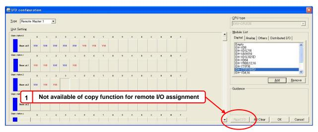
Figure 4.11 Example of I/O assignment for slave bases with Control editor (in system configuration example-1)
