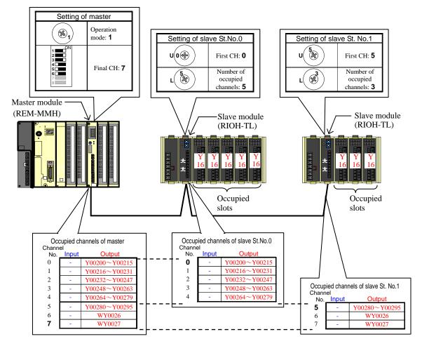
Figure 4.21 System configuration example-7 of Remote I/O MINI with mode-1
