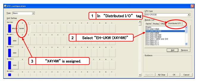
Figure 1.2 I/O assignment for remote master with control editor of unsupported version (in the case of "4W/4W")
