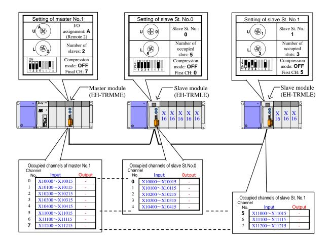
Figure 4.28 Replaced system configuration example-12 of the EH-150
