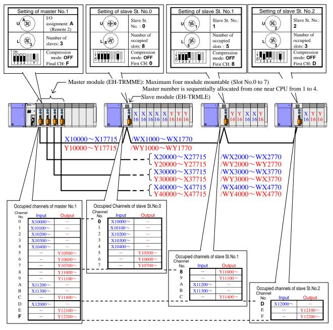
Figure 4.9 System configuration example-1 (I/O assignment of master: "Remote 2")
