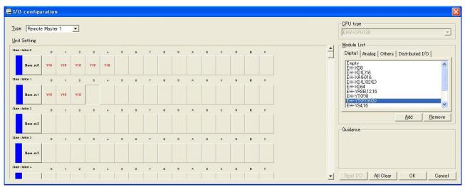
Figure 4.23 Example of I/O assignment for slave bases (with Control editor in system configuration example-8)
