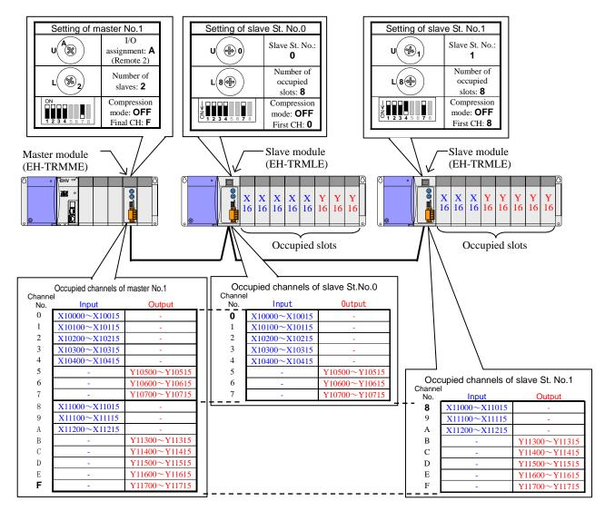
Figure 4.31 Replaced system configuration example-14 of the EH-150
