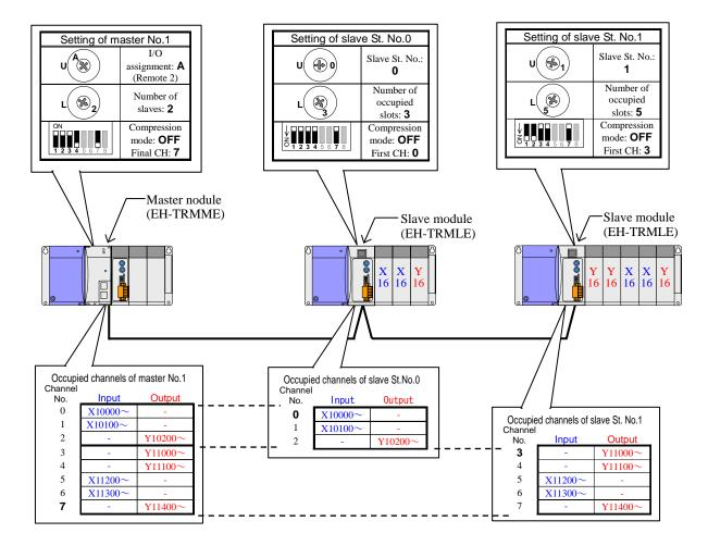
Figure 4.34 Replaced system configuration example-16 of the EH-150 with normal remote method
