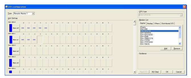
Figure 4.27 Example of I/O assignment for slave bases (with Control editor in system configuration example-12)
