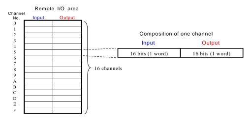
Figure 4.1 Composition of remote I/O area and one channel
