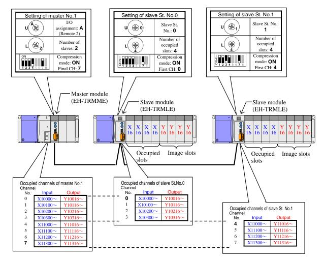
Figure 4.20 Replaced system configuration example-6 of the EH-150 (Using image slot)
