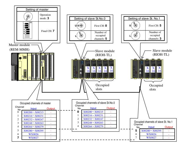
Figure 4.26 System configuration example-11 of Remote I/O MINI with mode-3
