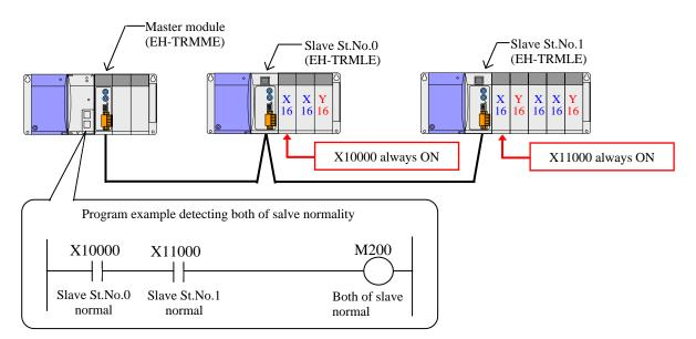
Figure 6.3 Slave abnormal detection method -1 (the case unnecessary of HOLD function)
