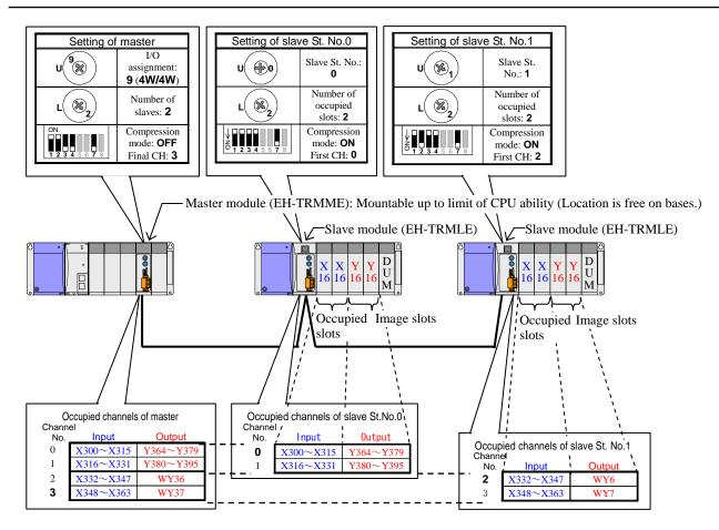
Figure 4.25 Replaced system configuration example-10 of the EH-150
