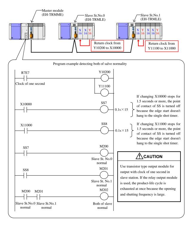
Figure 6.4 Slave abnormal detection method -2 (the case necessary of HOLD function)
