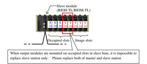
Figure 4.40 Impossible case of replacement with slave station only because output modules are mounted on occupied slots
