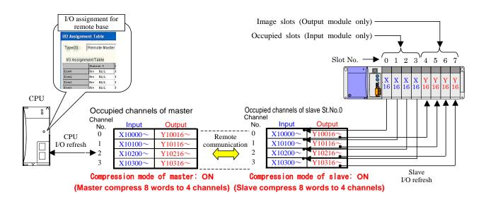
Figure 4.8 Correspondence of occupied channels and I/O slots (Compression remote method)
