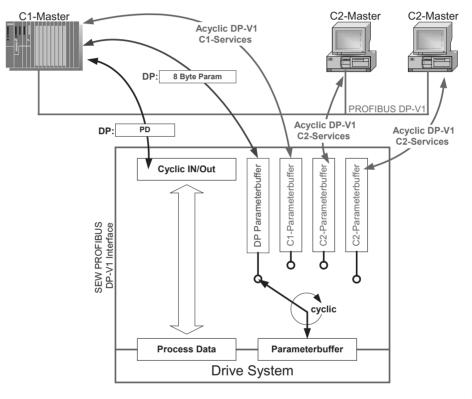
Figure 11: Parameter channels for PROFIBUS DP-V1
