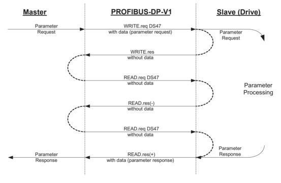
Figure 12: Telegram sequence for parameter access via PROFIBUSDP-V1
