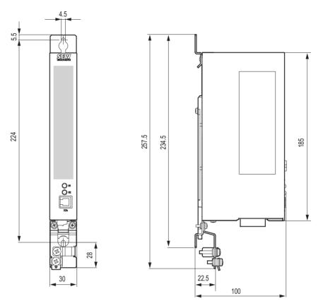
Figure 17: Device dimensions of the UOH11B gateway housing
