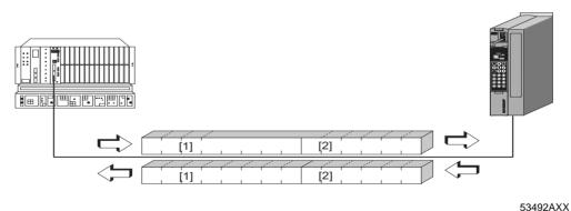
Figure 10: Communication via PROFIBUS DP
