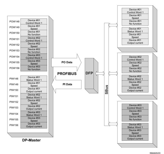
Figure 7: Data exchange DP-V1 master DFP inverter
