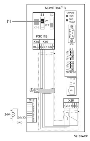
[1] Terminating resistor activated, S1 = ON
