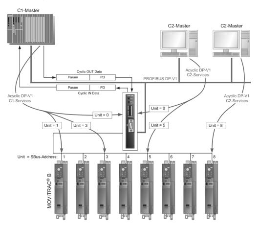
Figure 6: Data exchange with parameter data (Param) and process data (PD)
