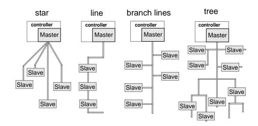
The maximum cable length for the total system may not exceed 100 m. By using 2 repeaters and additional AS-Interface power supplies, this can be extended to up to 300 m.
