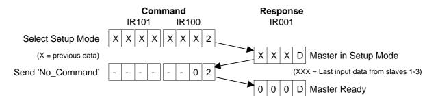
Note: It is also possible to select Setup Mode AND send 'No\_Command' in the same PLC scan by changing IR100 from XXX0 to XX02. The above method is safer if the output data of slave 1 needs to be held during execution of Setup Commands.
