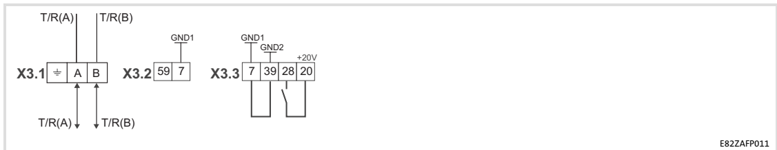
— The min. wiring requirements for operation
