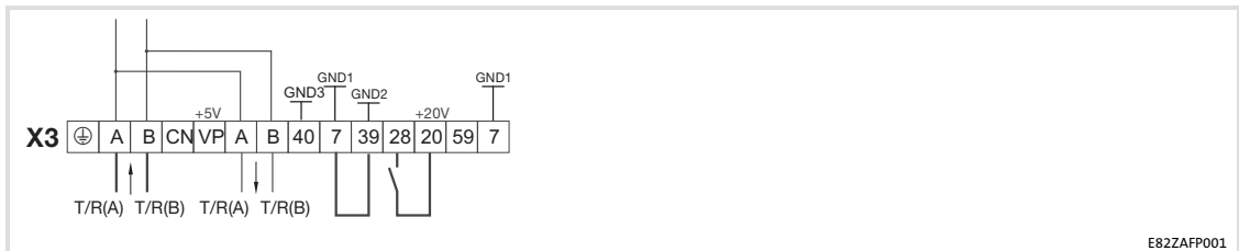
— The min. wiring requirements for operation
